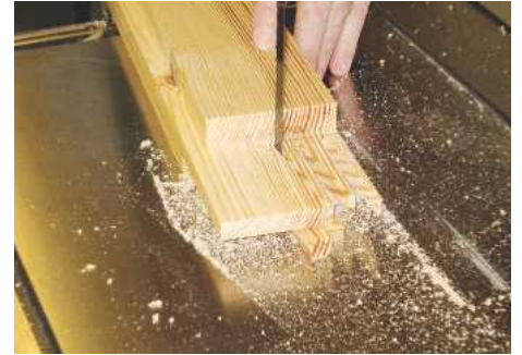
▲ Pic.5 The wedges themselves were cut from the waste material
